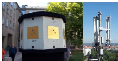
Figure 1. Transmit antenna (left) and receive antenna (right)
